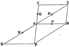
Lastly, let AB, AC represent any two forces P and Q, then shall the diagonal AD of the parallelogram ABDC represent the resultant in magnitude.
